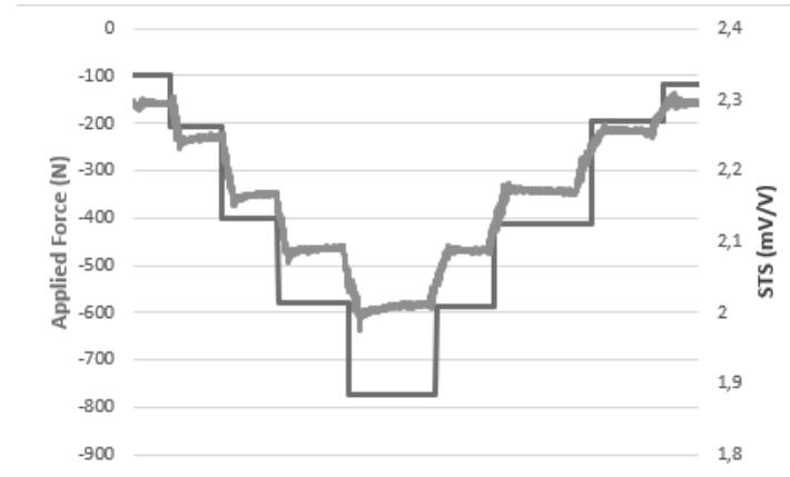
**Figure 1.9:** Example of tree pulling data: Tree 15, East gauge. The applied force (N) was recorded manually using a spring balance. The Strain Transducer Signal (STS, in mV/V) is the strain gauge reaction during the tree pulling. The curves are reversed because for practical reasons the tree has been pulled on the opposite side to the strain gauge.
