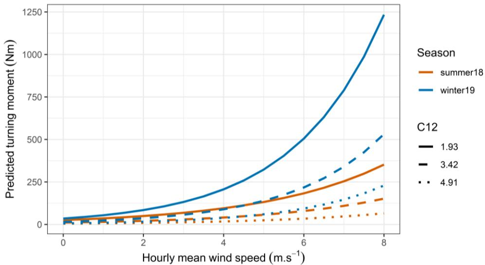
**Figure 2.4:** Predicted turning moment during winter and summer as a function of  $C_{12}$ .
