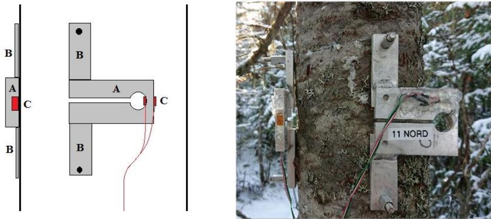
**Figure 1.7:** Sensors fixed on a balsam fir, following the design of Moore et al. (2005). With A the aluminum bracket; B the two anchor wings; and C the two strain gauges glued on the bracket.
