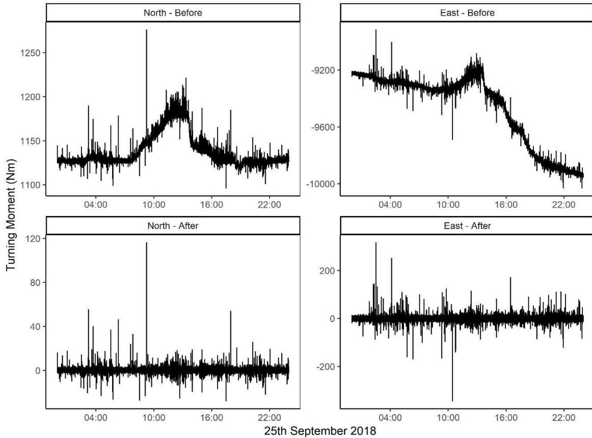
**Figure 1.10:** North and East gauges of Tree 15 for the 25th September 2018, before and after the use of the Butterworth filter (Butterworth, 1930).
