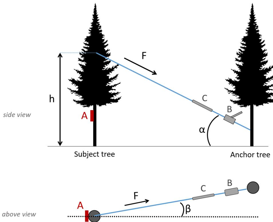
**Figure 1.8:** Sensor calibration diagram. With A the sensor to calibrate; B the manual winch; C the spring balance; F the force applied ; h the attachment height ;  $\alpha$  the angle of winching ; and  $\beta$  the anchorage deviation angle, based on Wellpott (2008).
