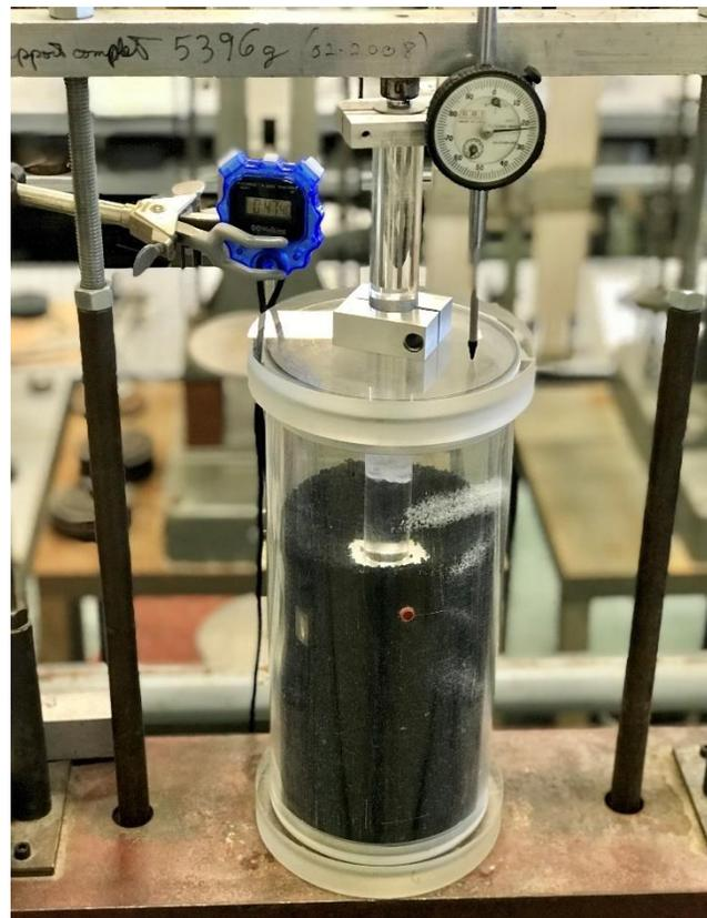
**Figure 3.24** Rigid circular plate resting on a TDA-sand mixture
