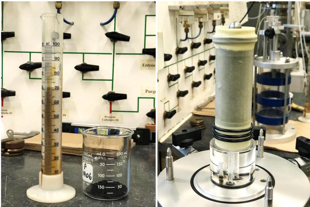
**Figure 2.12** Test materials (sand and TDA) and triaxial test sample preparation
