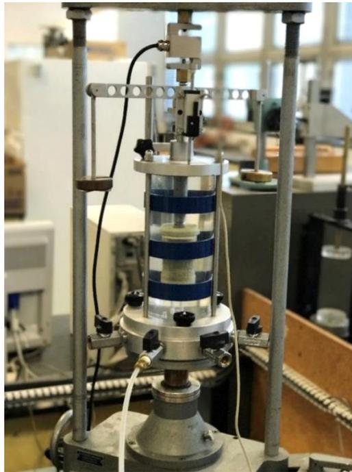
**Figure 4.3** Triaxial test configuration
