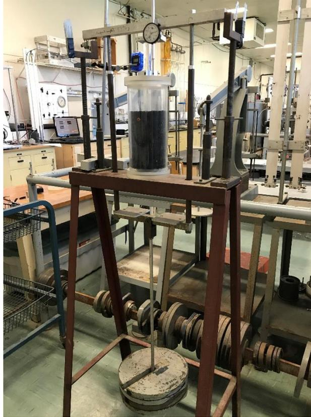
**Figure 3.25** Laboratory setup for small-scale circular rigid plate resting on a TDA–sand mixture
