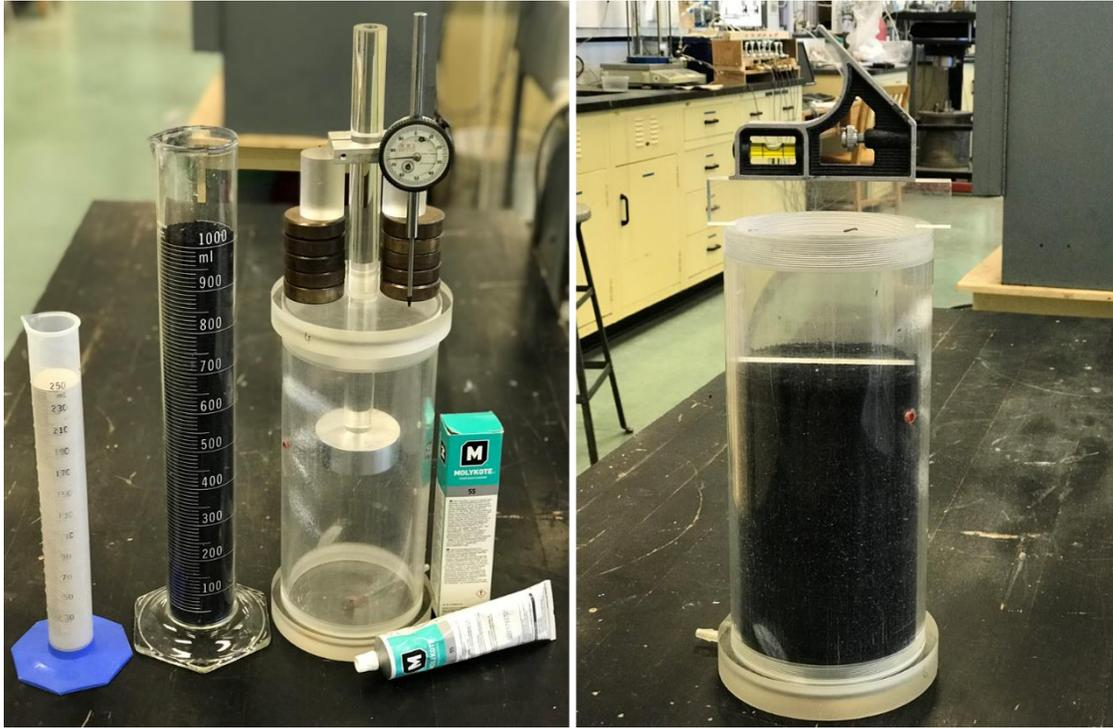
**Figure 2.18** Test materials (sand and TDA) and the testing cell before and after the sample preparation and placement
