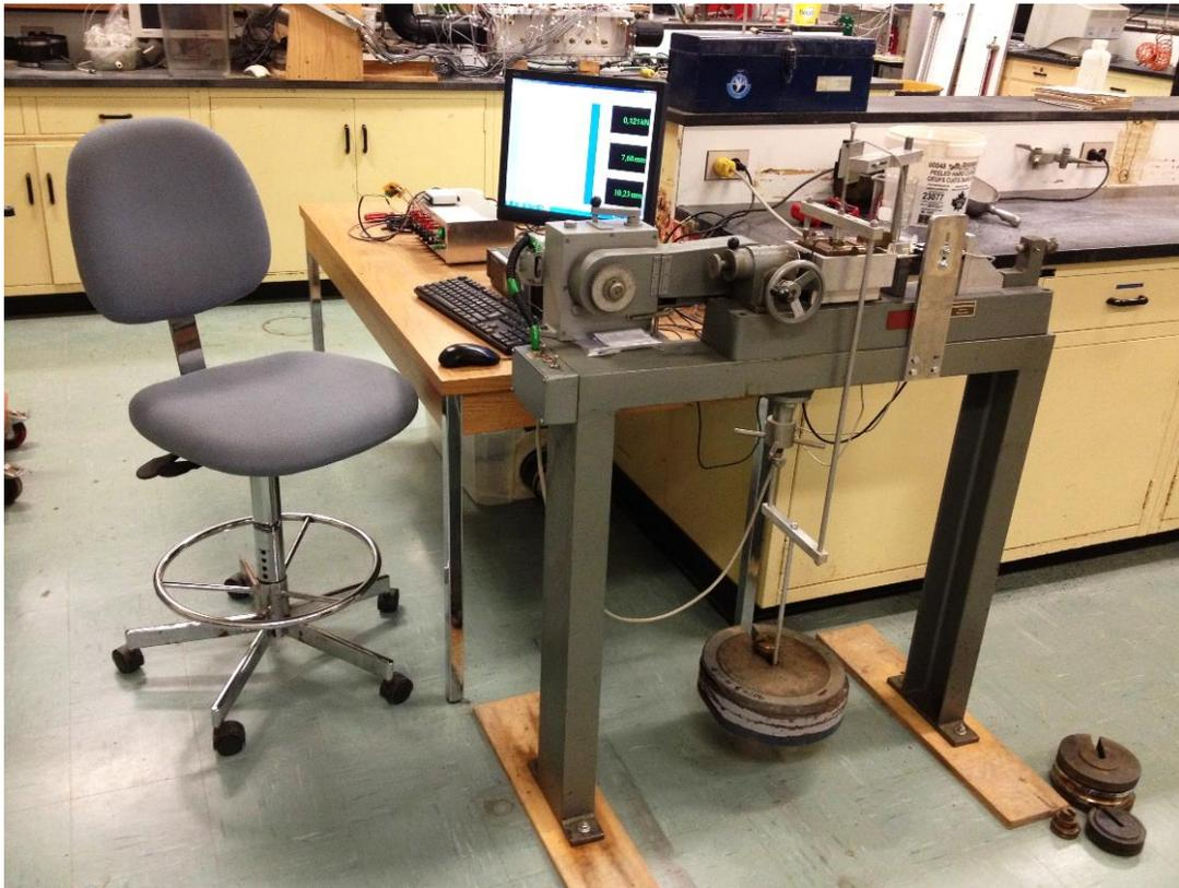
**Figure 3.5** Typical shear box test setup to determine the friction angle between TDA–soil mixture and aluminum alloy 6061
