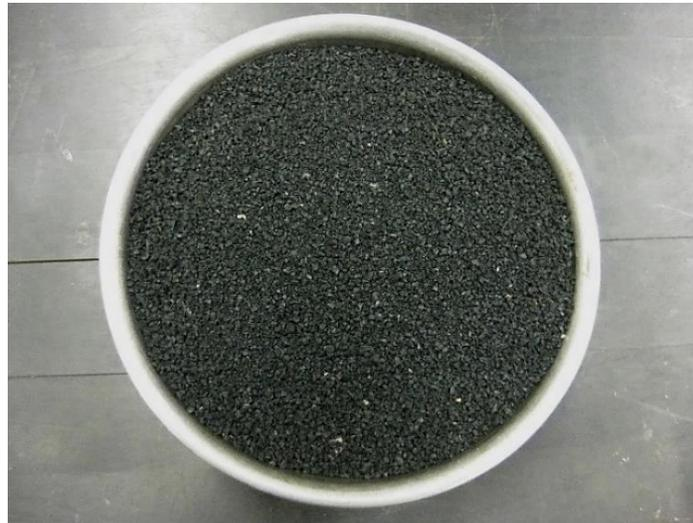
**Figure 2.1** TDA granular material employed in this study
