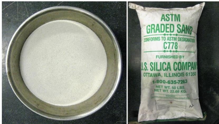
**Figure 2.4** Graded Ottawa sand used in this study
