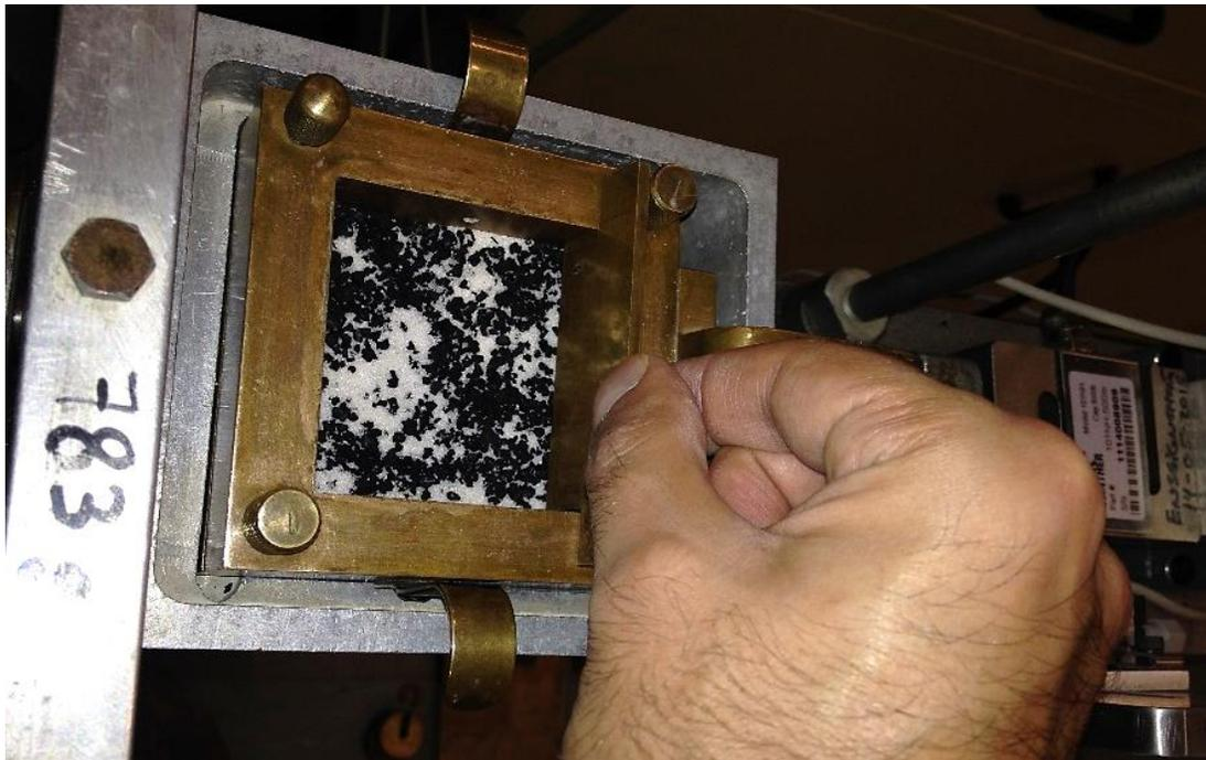
**Figure 2.17** Flattening of surface of the sample before placement of the loading cap
